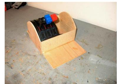
Here's the completed assembly with a test fit for function of the unit. You can see here the levers are now at a realistic angle and the buttons are much easier to reach.
