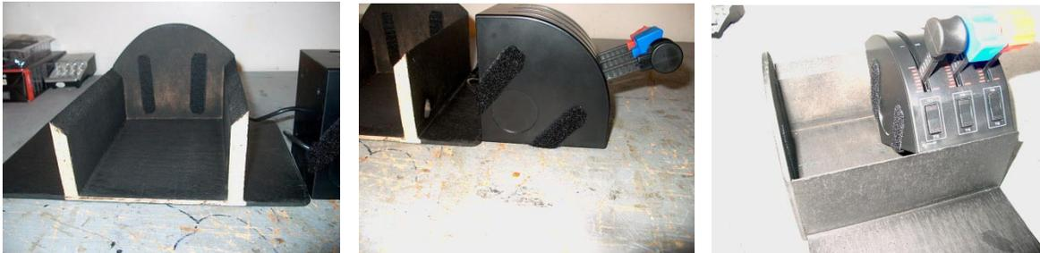
I used velcro to hold the unit snugly to the side of the adapter and eliminate any sloppiness in the control movement. When another throttle quadrant is installed the other end plate can be adjusted to secure both units snugly against each other.
